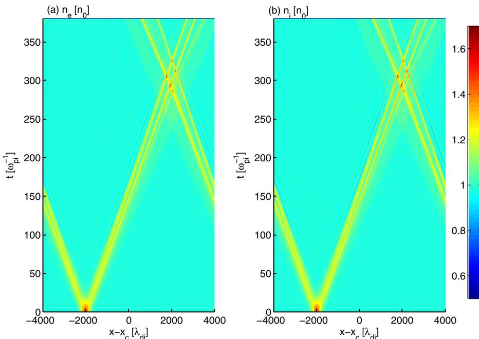
FIG. 2. Spatio-temporal evolution of the densities of the electrons and ions in the simulation.
