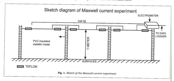
Let us consider a steady state, we assume  $\mathbf{i} = \mathbf{I}_{\mathrm{m}} \sin(\omega t)$ , and the charge  $q = \frac{Q_{\mathrm{0}} - I_{\mathrm{m}} \cos(\omega t)}{\omega}$  where  $\mathbf{I}_{\mathrm{m}}$  is the maximum amplitude of the AC current and  $\mathbf{Q}_{\mathrm{0}}$  is the constant of charge accumulation on the wire of the capacitor.
