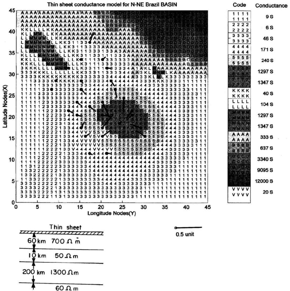
Fig. 5. Thin sheet conductance map for the Basin model. Conductance codes and their conductance values, as defined in Table 1, are also indicated. Gray shades distinguish zones of different conductances. Resulting response at the 12 min period is shown by the induction arrows only for the nodes representing the magnetometer sites. Also shown at the bottom is the layered structure beneath the thin sheet.
