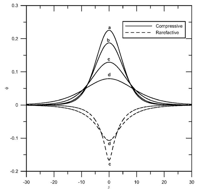
FIG. 3. Variation of potential  $\phi$  with  $\xi$  for different electron beam velocities: (a)  $u_0=0.3$ , (b)  $u_0=0.4$ , (c)  $u_0=0.5$ , and (d)  $u_0=0.55$ . Other parameters are:  $Ma=1.1$ ,  $\mu=0.2$ ,  $\alpha=0.06$ ,  $\beta=0.01$ .
