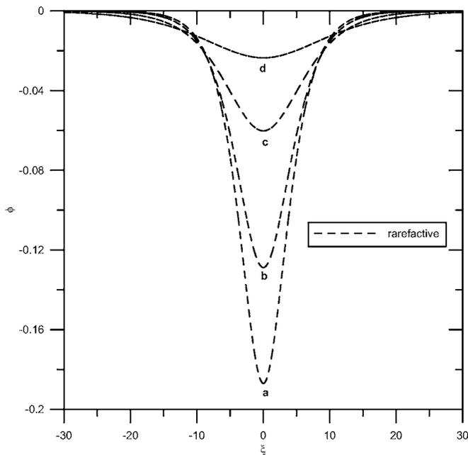
FIG. 1. Variation of potential  $\phi$  with  $\xi$  for different electron beam velocities: (a)  $u_0=0.3$ , (b)  $u_0=0.4$ , (c)  $u_0=0.5$ , and (d)  $u_0=0.55$ . Other parameters are:  $Ma=1.1$ ,  $\mu=0.0$ ,  $\alpha=0.06$ ,  $\beta=1$ .
