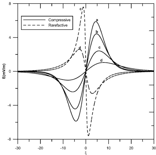
FIG. 4. Variation of electric field  $E$  with  $\xi$  for different electron beam velocities: (a)  $u_0=0.3$ , (b)  $u_0=0.4$ , (c)  $u_0=0.5$ , and (d)  $u_0=0.55$ . Here  $T_l=5$  eV,  $n_0=0.1$  cm $^{-3}$ , and other parameters are same as used in Fig. 3.
