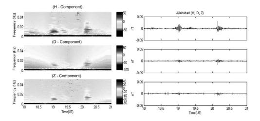
**Figure 1.** Typical Pc4 pulsations as observed on 01 April 2005. The left panel is the dynamic spectra of X (N-S),Y(E-W) and Z (Vertical) components of geomagnetic field variations and the right panel shows the corresponding temporal variations.
