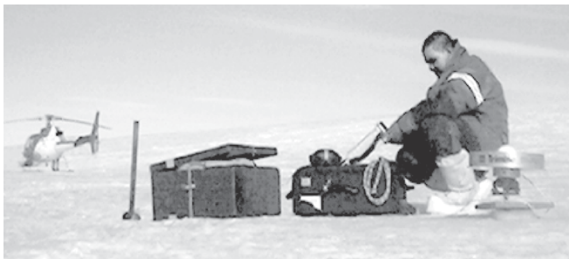
Fig. 2. GPS antenna mounted on wooden platform and GPS receiver being set for the collection of GPS data at Schirmacher glacier.
