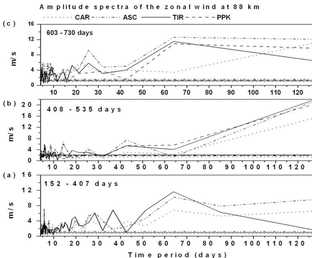
**Figure 3.** Amplitude spectra of the daily zonal winds at 88 km over four sites for the three time intervals (a) 152–407 days, (b) 408–535 days, and (c) 603–730 days. The horizontal lines represent the 95% confidence levels.
