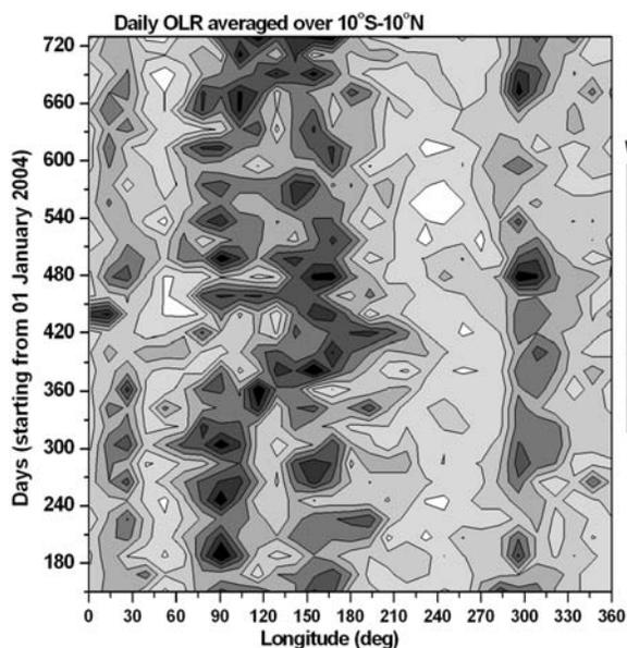
**Figure 7.** Time-longitude cross sections of the OLR ( $\text{W/m}^2$ ) averaged over  $10^\circ\text{N}$ – $10^\circ\text{S}$  for the observational period 1 June 2004 to 31 December 2005.
