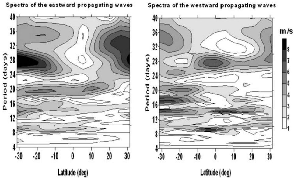
**Figure 13.** Amplitude spectra of the (left) eastward and (right) westward traveling waves with zonal wave number 1 in Met Office zonal winds (m/s) at pressure level 0.1 hPa for the observational period 1 June 2004 to 31 December 2005.
