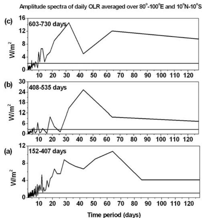
**Figure 8.** Amplitude spectra of the daily OLR averaged over  $80^\circ\text{E}$ – $100^\circ\text{E}$  and  $10^\circ\text{S}$ – $10^\circ\text{N}$  region for the three time intervals (a) 152–407 days, (b) 408–535 days, and (c) 603–730 days. The horizontal lines represent the 95% confidence levels.
