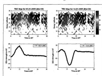
**Fig.1(a-b).** Shows the day-to-day variability in the EEJ strength and its associated changes in the GPS TEC obtained on 05-01-2006 and 14-01-2006.
