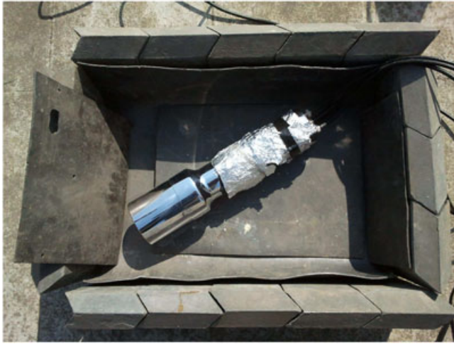
Figure 3. Top view of NaI(Tl) scintillation detector used for the observations, which was kept inside lead shielding.
