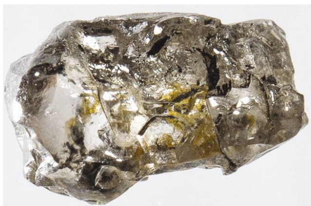
Figure 1. Enlarged image of impure diamond from Juína, Brazil (courtesy: Graham Pearson, University of Alberta). The diamond is 5 mm in long axis. A microscopic inclusion of ringwoodite, which is a high-pressure polymorph of mineral olivine [(Mg,Fe) 2 SiO 4 ] was documented using Raman spectroscopy by Pearson et al. 1 .
