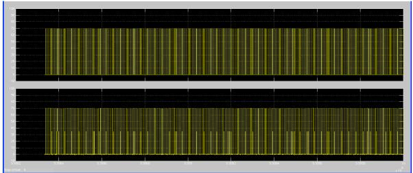
Fig -5: Signal amplitude measurement above scope shows sending end amplitude in db, below scope shows receiving end amplitude in db.
