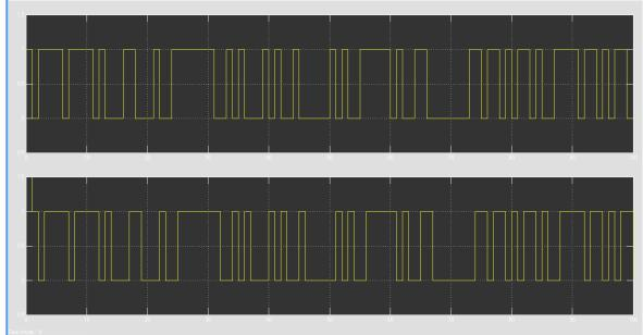
Fig -4: Bit delay, above transmit end bit scope, below receive end bit scope. Time is in micro second.
