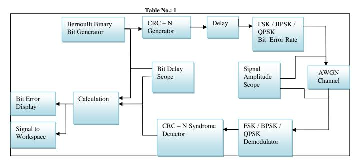
Fig-2: Block diagram of digital modulation communication system.
