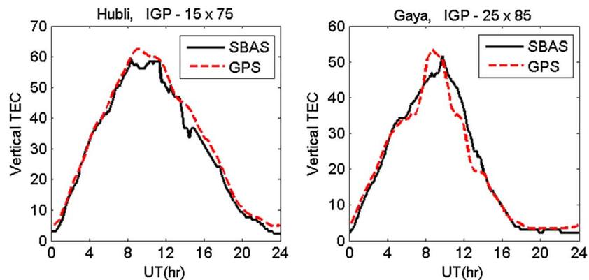
**Figure 8.** Comparison of vertical TEC derived from GPS measurements (dashed line) and SBAS (GAGAN) corrections (solid line) at two different locations—(left) Hubli (15.3°N, 75°E) and (right) Gaya (24.75°N, 84.95°E) on a typical day of 23 November 2012.
