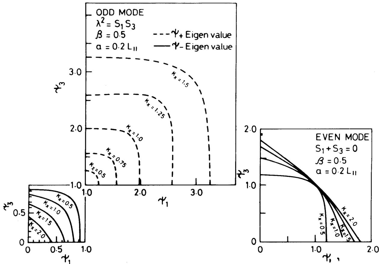
Fig. 2— $\psi_3$  versus  $\psi_1$ , for different values of  $k_x$ . For the case where  $S_1 + S_3 = 0$ , there is only one set of graphs. But there are two sets of graphs corresponding to  $\psi_+$  and  $\psi_-$  when  $\lambda^2 = S_1 S_3$ .
