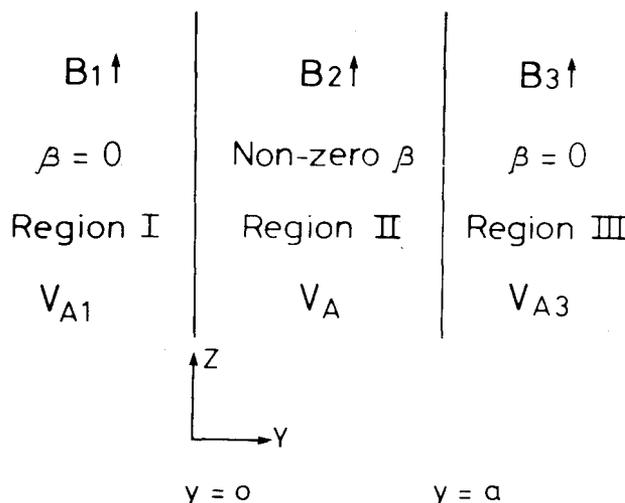
Fig. 1—Model of a hot surface layer of thickness  $a$  between two cold media.
