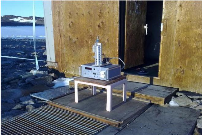
Figure 2: Photograph of the Quartz Crystal Microbalance Impactor. The sensing stack is kept over the control unit.
