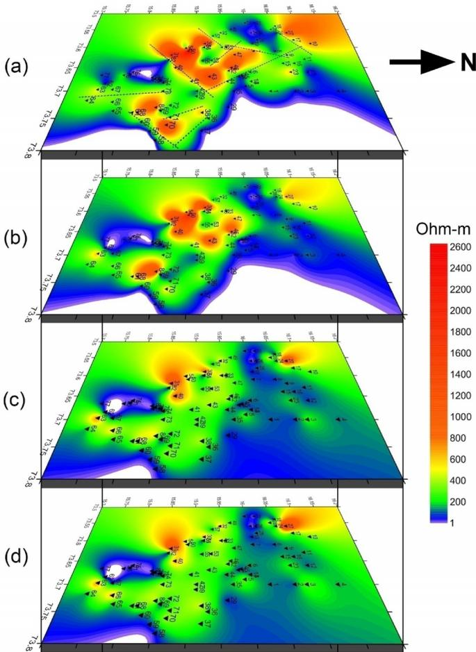
**Fig. 5.** Apparent resistivity surface map at different depths (a) at depth = 2 m (b) at depth = 5 m (c) at depth = 15 m (d) at depth = 20 m
