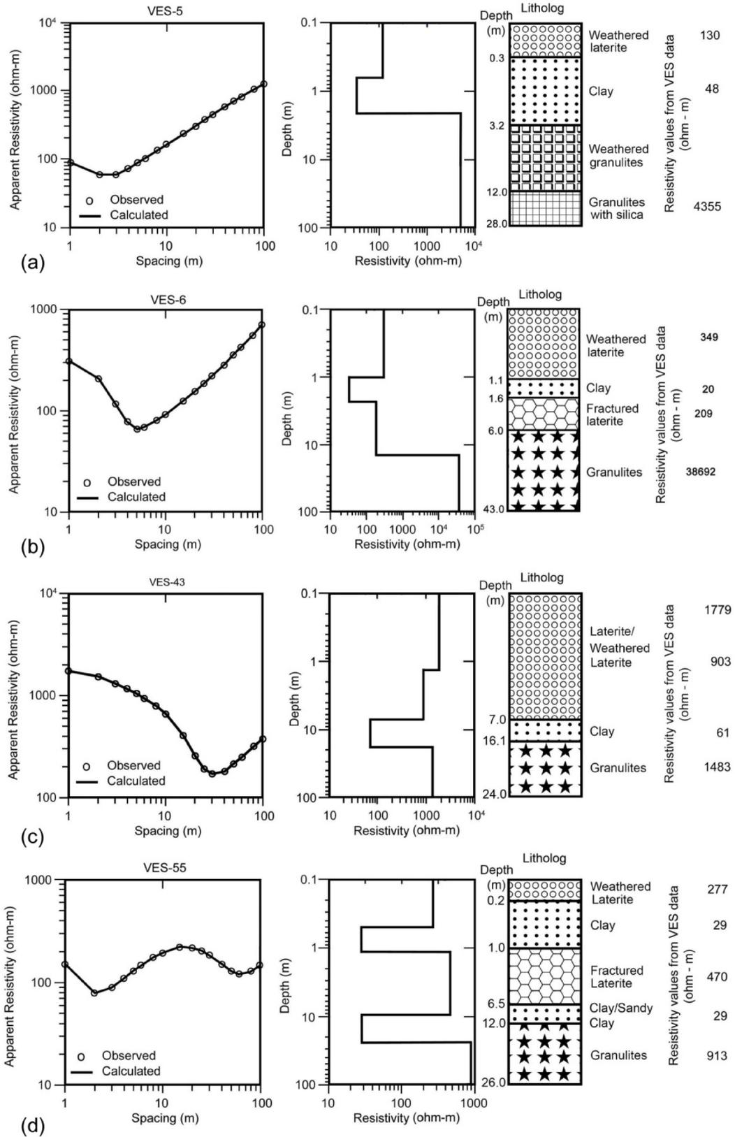
**Fig. 2.** Vertical electrical sounding curves and inversion results at **(a)** VES 5 **(b)** VES 6 **(c)** VES 43 **(d)** VES 55. Also, the correlation of borehole lithology with the corresponding resistivity values obtained from VES data is shown.
