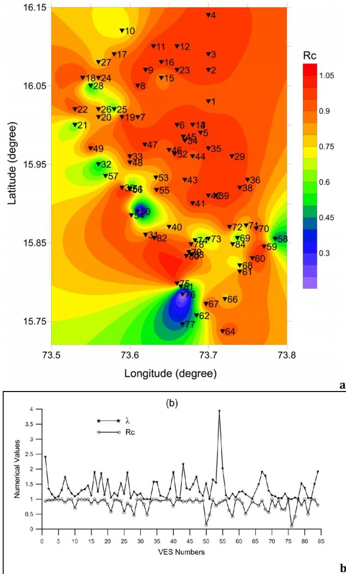
Fig. 4. (a) Spatial variation of reflection coefficient in the study area. (b) Plot of coefficient of anisotropy ( $\lambda$ ) and reflection coefficient (Rc) with VES number.
