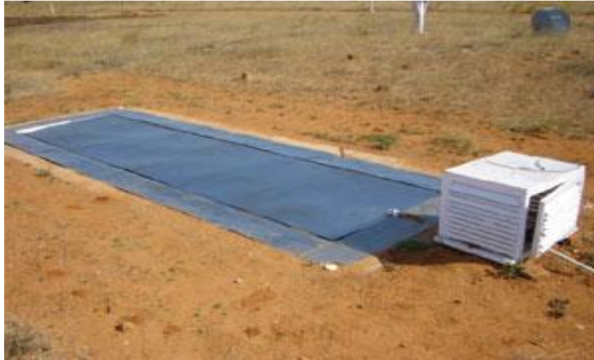
Fig. 3. 4. Photograph of Wilson's Plate antenna
