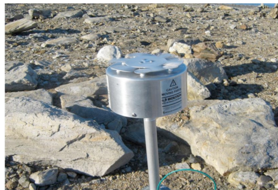
Fig. 2. Photograph of Electric Field Meter-100.
