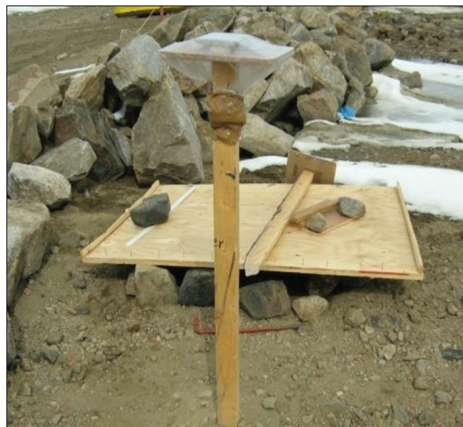
Figure 2: Photograph showing the deployment of passive dosimeters at Antarctica at a height of 1 m from ground on a wooden plank
