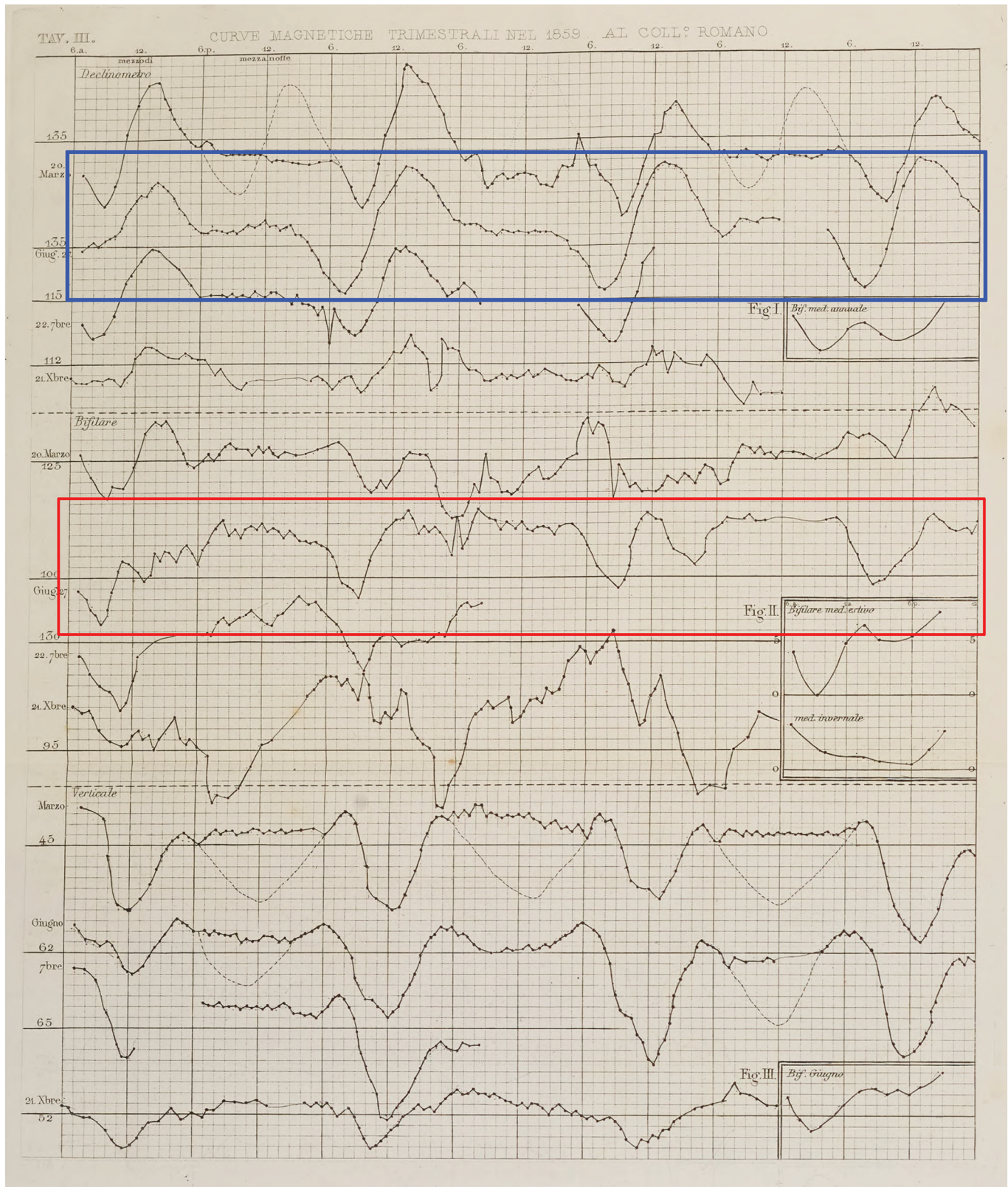
Figure 1. Measurements taken at the Rome Observatory during 1859. The time series are for a declinometer (top), two-wire magnetometer (middle), and vertical magnetometer (bottom). The blue and red boxes enclose the declinometer and horizontal measurements taken for 27–30 June 1859. From Secchi (1859b).
